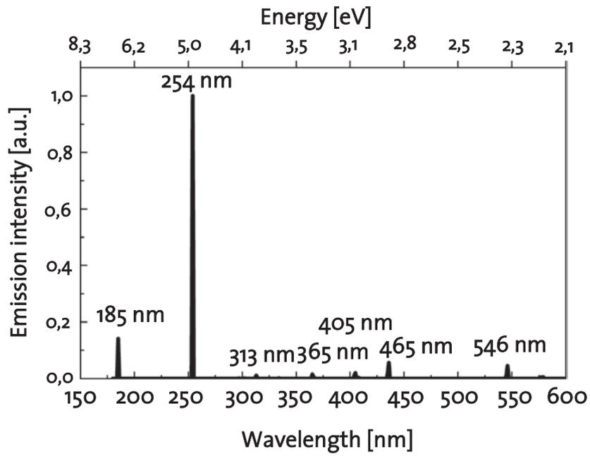
Figure 2 Emission spectrum of a typical Hg medium pressure lamp (source: own representation).
