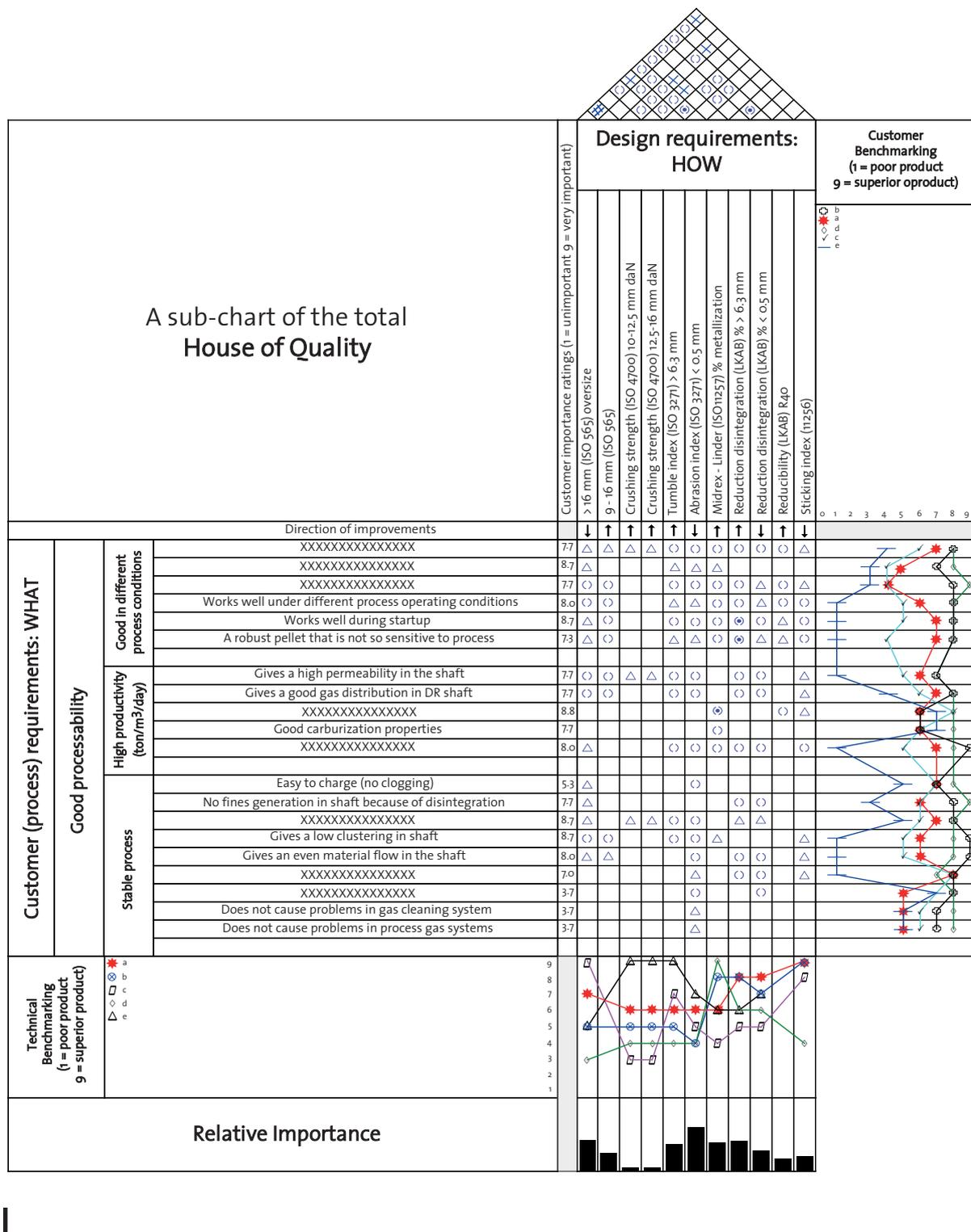
room rather important. This can also be seen in the roof of figure 5. Since the relation between the design requirements “tumble index” and “abrasion index” is strongly positive, an improvement of the “tumble index” will automatically show a decrease in the “abrasion index”, which is very positive since the disintegration of pellets is not wanted.
